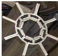
Each individual Frac Initiated & Propagated by Dedicated Tubing to Dilating Cavities in Production Version of STAR Frac Casing
