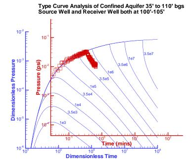
FIGURE 4. Type Curve Match for Hydraulic Pulse Interference Test.
