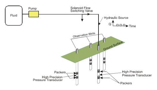
FIGURE 1. Point Source Hydraulic Pulse Interference Test
