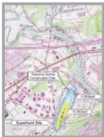
Contaminated Groundwater Plume
