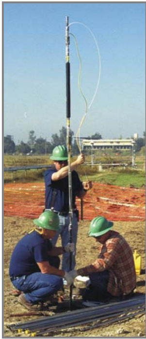
Sam Wells, Chad Givens and Chris Givens Setting Up The Hydraulic Pulse Interference Test
