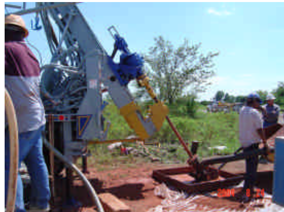
Figure 4. Inclined Magnetometer Profiling to verify PRB thickness
