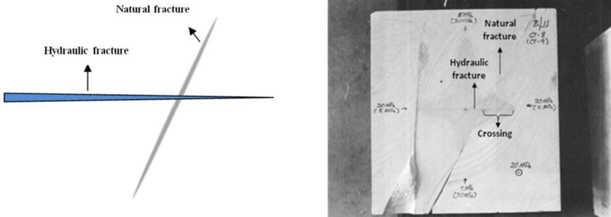
**Figure 2a. Propagating hydraulic fracture crosses the natural fracture and keeps propagating without any significant change. Left is a schematic and right is experimental study from Blanton (1982).**
