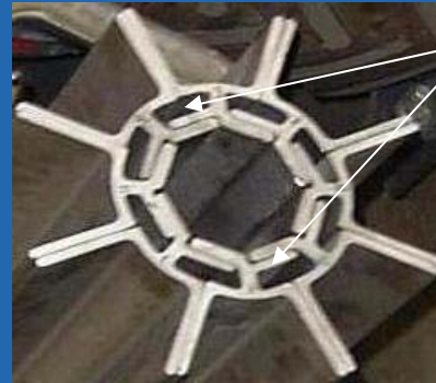
Diametrically Opposite Cavities are Dilated to Initiate Azimuth Controlled Vertical Planes
